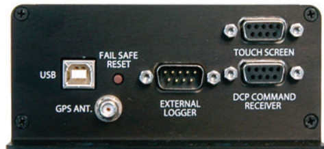
Stevens SatComm Transmitter (front panel) Stevens Part #93876
