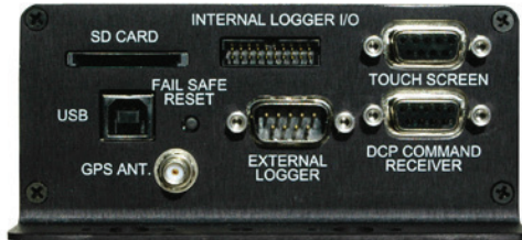
Stevens SatComm Transmitter with Data Logger (front panel) - Stevens Part #93876-001
